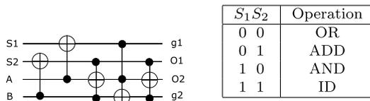
**Fig. 13** Mini-ALU: Minimum MCT circuit and its operation assignment.
