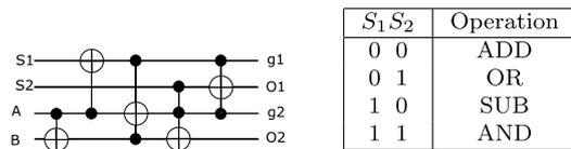
**Fig. 15** ALU: Minimum MCT circuit and its operation assignment.
