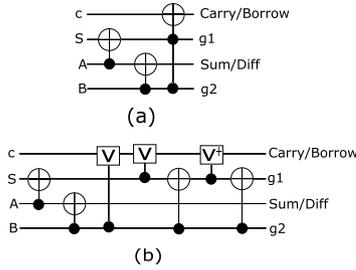
**Fig. 11** The proposed half adder/subtractor: (a) the minimum MCT circuit, and (b) the reduced quantum circuit.
