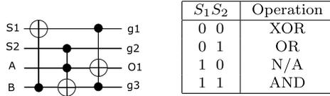
Fig. 16 LU: Minimum MCT circuit and its operation assignment.
