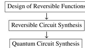
Fig. 1 Overview of the design flow of reversible synthesis.
