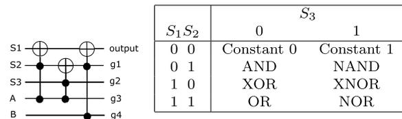
**Fig. 14** Gupta's-LU: Minimum MCT circuit and its operation assignment.
