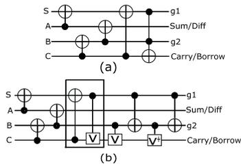
**Fig. 12** Proposed full adder/subtractor (a) minimum MCT circuit, and (b) reduced quantum circuit.
